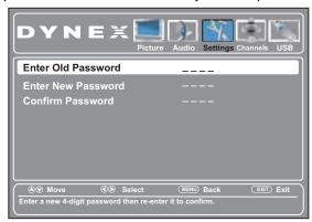
**6** Press the number buttons to enter the old password, then enter a new password. On the next line, enter the new password again to confirm it. The *Parental Controls* menu opens again.
